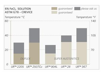
The high chromium, molybdenum and nitrogen contents of alloy  $UR^{\mathbb{M}}$  367 (PREN > 43) explain why the grade is very resistant to localized corrosion even in acidified oxidizing environments. The alloy has been used for seawater applications.
