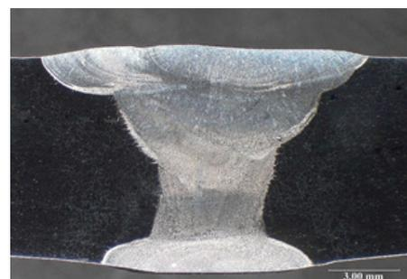
Micrographic view of a UR™ 32615 welded sample
