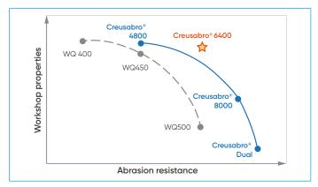
**Creusabro® 6400** has been developed to meet all situation where improved wear resistance is required keeping the same formability and easy process-ability in the workshop as classical 450 HB plates.
