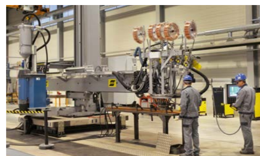
Welding laboratory: Multi-wire Submerged Arc Welding (SAW)
