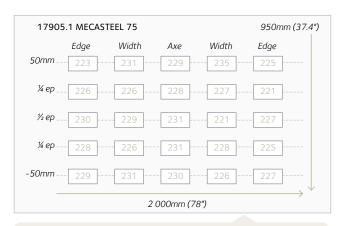
Hardness homogeneity through a 950 mm thick block Mecasteel 75 (237 HB max).
