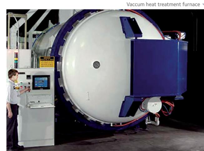
Similar heat treatment process can be applied to both ISOTROP and H13
