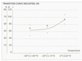
Typical value measured 2,5" below the skin of a block 30.7" (780 mm) thick
