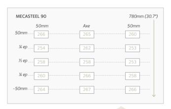
Hardness homogeneity of a 780 mm / 30.7" thick block Mescasteel 90.
