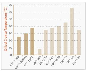
Thanks to its chromium, molybdenum, tungsten and nitrogen contents, UR™ 66 presents an excellent resistance to localized corrosion, much better than conventional 6%Mo and 7%Mo grades, and 625 alloy when tested according to the most common standards.
