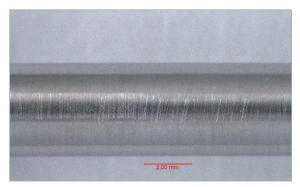
UR<sup>™</sup> 4565 after 720 hours (7 bar  $H_2$ S, 250 g/l NaCl, pH 4.5, 150°C) at 90%AYS
