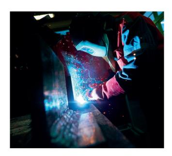
UR™ 4565 can be welded with niobium free base filler material ER Ni.Cr.Mo-7 or EN Ni.Cr.Mo-10 (AWS A5.14) wire, and E Ni.Cr.Mo-7 or E.Ni.Cr.Mo-10 (AWS A 5.11) electrodes or filler metal as EL Ni.Cr.19 Mo-15 or SG Ni.Cr.20 Mo-15; EL Ni.Cr.23.Mo-16 or SG Ni.Cr.23 Mo-16 (DIN 1736) electrodes or filler metal can also be used. Suitable electrodes and welding wire are available from various suppliers. Technical assistance is available upon request.
