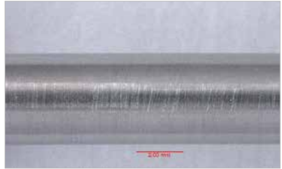
UR™ 4565 after 720 hours (7 bar H 2 S, 250 g/l NaCl, pH 4.5, 150°C) at 90%AYS
