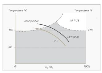
In most of the corrosive solutions, alloy  $UR^{TM}$  28 is more corrosion resistant than alloy  $UR^{TM}$  904L (N08904). The alloy is extensively used in phosphoric acid applications and some sulphuric solutions. Alloy  $UR^{TM}$  28 may also be used in caustic solutions since its molybdenum content remains low comparing with the nickel and chromium additions.
