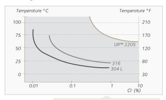
Sensitivity to pitting corrosion. Effects of temperature and chloride content
