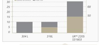
Depassivation conditions of several stainless steels Solution: 30 g/l NaCl 20°C
