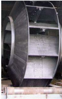
Extra large fans (XXL), extreme service conditions (blade protection)
