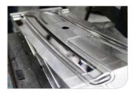
Orange peel on a mould cavity
