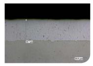
Micrograph of hard chrome plated layer (hardness: 970 HV0.1 Kgf)
