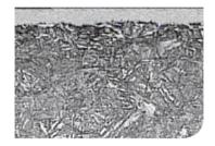
Typical micrograph of a gas nitriding layer
