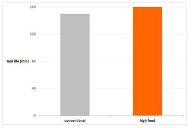
Milling tool life for conventional and high feed milling
