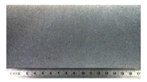
Macrograph of Superplast® 2738mod (acid test)
