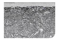
Typical micrograph of a gas nitriding layer
