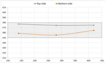
Brinell hardness profile through 560mm-thick blocks
