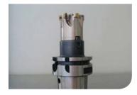
Conventionnal milling (SECO tools) cutter : R220.29-0040-06.4A insert : RPHT 1204MOT-M15 High feed milling (SECO tools) cutter : R220.21-0040-LP06.6A insert : LPHW 1204MOT-D06
