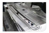
Orange peel on a mould cavity
