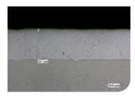
Micrograph of hard chrome plated layer (hardness: 970 HV0.1 Kqf)
