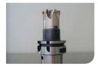
Conventionnal milling (SECO tools) High feed milling (SECO tools) cutter: R220.29-0040-06.4A insert : RPHT 1204MOT-M15
