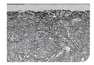
Typical micrograph of a gas nitriding layer
