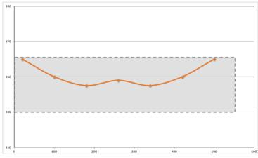
Brinell hardness profile through 540mm-thick block
