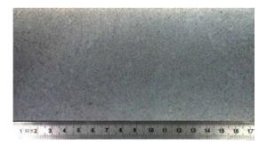
Macrograph of Superplast® 2738mod HH (acid test)
