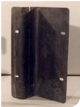
*Example of part obtained after cold bending.
