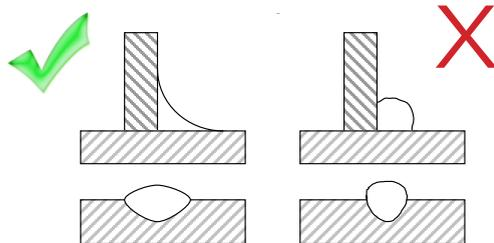
Particular case: At the ends of seams, crater cracks may occur. Thus it may be necessary to modify the parameters for arc fading in order to feed the crater at the end of the seam (here a convex form is preferred).
