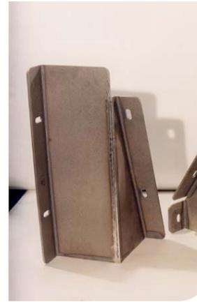
Part obtained by laser welding. Mars® 500 steel
