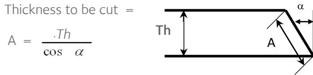
The maximum thickness is thus based on the thickness of the plate and the bevel.
