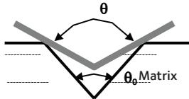
When the mandrel raises, the bend opens to an angle  $\Theta$ .
