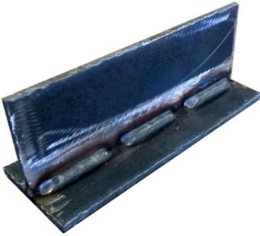
T (MIG) Assembly: test performed at the Centre de Recherche Industeel, Mars® grade 600, thickness 8.4 mm (0.33")
