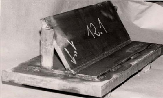
Assembly with a coated electrode performed at the Centre de Recherche Industeel, Mars® grade 240
