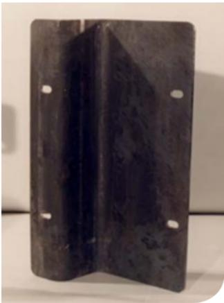
*Example of part obtained after cold bending.*
