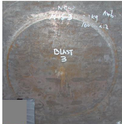
Mars® 220 sample th15 mm (.6") after blast test (classified results)
