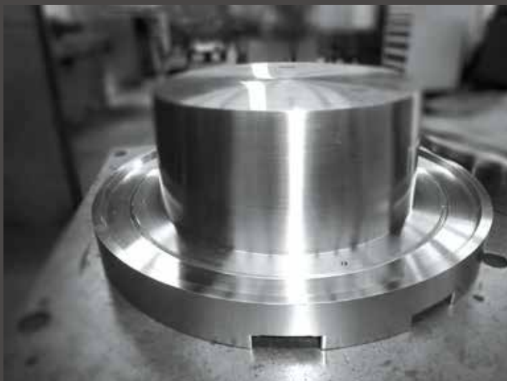
Rubber mould component after machining ▲
