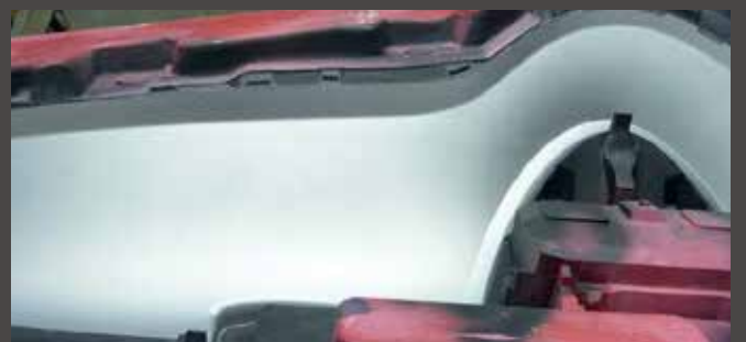
Cavity made of Superplast® 2738mod. was approved by end user
