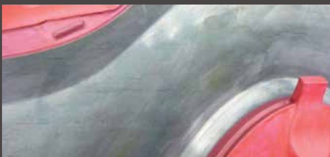
Cavity made of standard W 1.2738 was rejected due to segregation streaks
