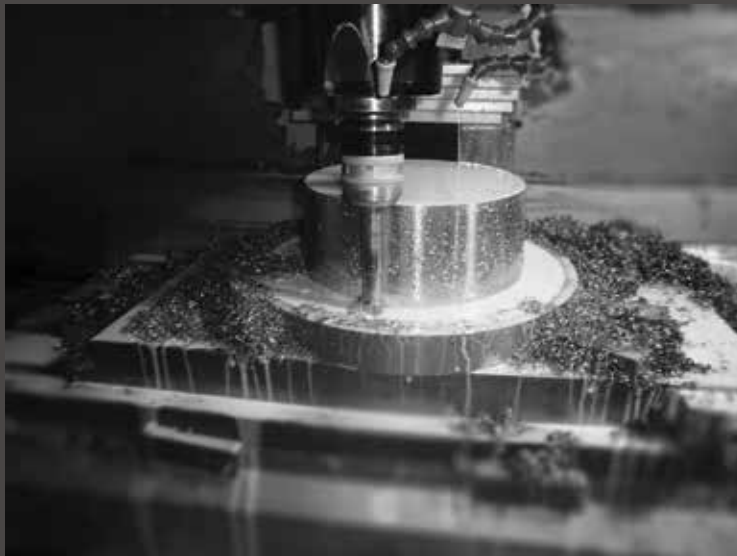
Rough machining of Superplast® 2738mod. plate ▲
