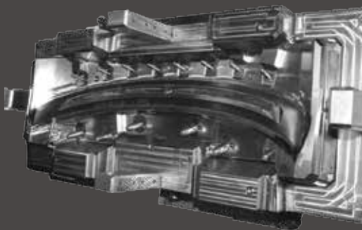
Front grid mould in Superplast® 400 ▼
