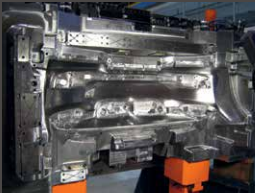
Front bumper cavity in Superplast® 2738 mod. ▼
