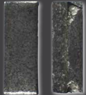
▲ Comparison between Creusabro DUAL (left) and Chromium Carbide Overlay (right) specimens exposed to impact wear. No chipping to be seen!
