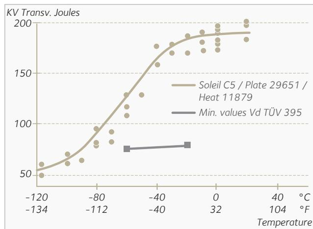
Soleil™ C5 alloy presents improved toughness properties when compared to ferritic-martensitic grades (AISI 410- 420 / EN 1.4000-X6 Cr 13).
