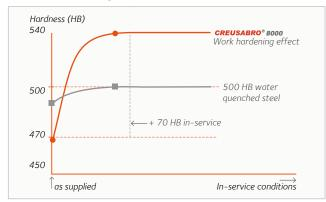
In addition, the super ductility of the retained austenite contributes to improve the lifetime in service by allowing larger micro shearing and thus delays the ultimate tearing of metal particles from the surface of the material exposed to the abrasive.
