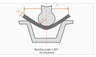
According above parameters, bending strength depends on bending length, thickness, die opening...
