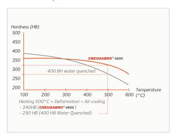
These properties enable the steel to be processed in the hot condition 450 - 500°C (840 - 930°F): forming of thick plates, for example, followed by a slow cooling without inducing any significant drop of hardness. Hot resistance of Creusabro° 4800 allows its use in hot environments where pieces are heated up to 350°C (660°F).
