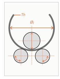
**Creusabro**° **4800** can be hot formed at a temperature of 450 - 500°C (840 - 930°F) without any further heat treatment. At this temperature the force necessary to deform the plate will be lower than at room temperature, and the deformation capability of the steel will be higher (smaller forming radius).
