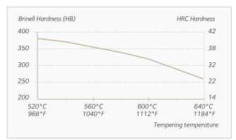
Note that complicated shapes require accurate control of steel temperature uniformity and sufficient holding
