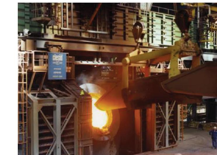
Metal scraps Feeder in ArcelorMittal Fos, use of Creusabro® 8000 allows weight reduction and reduce energy consumption
