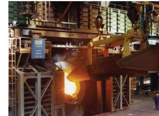
Metal scraps Feeder in ArcelorMittal Fos, use of **Creusabro® 8000** allows weight reduction and reduce energy consumption
