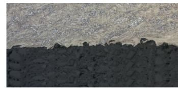
Sample aspect after 2h MLD test, 150 beats (3J)/min, 200 rot/min, Silica flow 7,12 g/s
