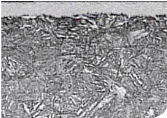
Typical micrograph of a gas nitriding layer
