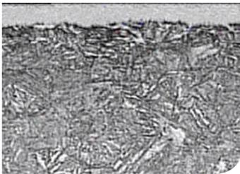
Typical micrograph of a gas nitriding layer
