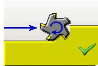
Climb milling (down milling)
