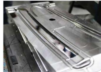
Orange peel on a mould cavity
