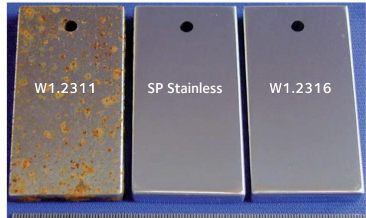
Sample following corrosion resistance test
