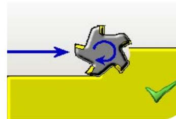
Climb milling (down milling)
