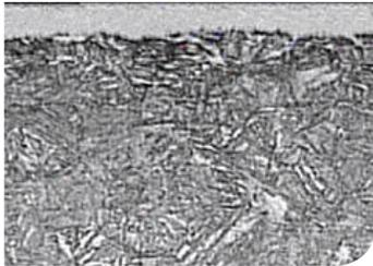
Typical micrograph of a gas nitriding layer
