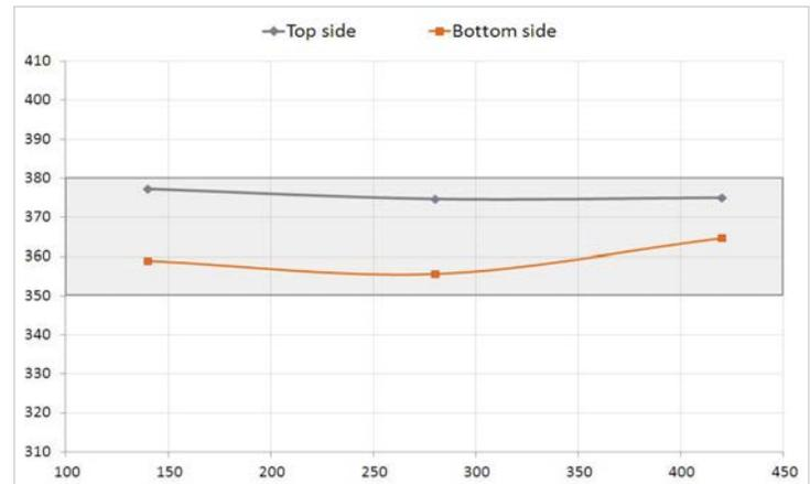
Brinell hardness profile through 560mm-thick blocks
