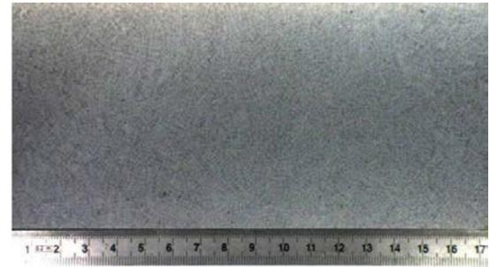
Macrograph of Superplast® 2738mod HH (acid test)
