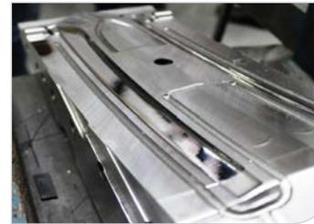
Orange peel on a mould cavity
