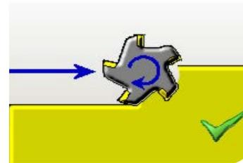
Climb milling (down milling)
