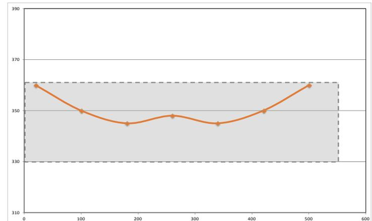
Brinell hardness profile through 540mm-thick block
