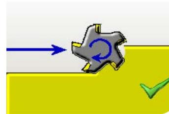
Climb milling (down milling)
