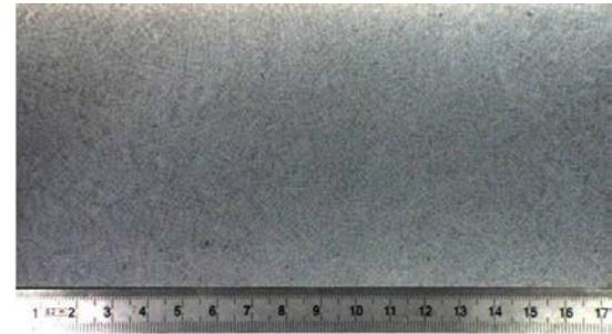
Macrograph of Superplast® 2738mod (acid test)
