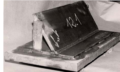
Assembly with a coated electrode performed at the Centre de Recherche Industeel, Mars® grade 500
