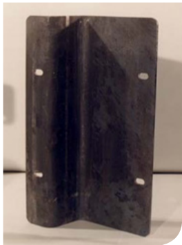
Example of part obtained after cold bending. Mars® 500 steel Th 4.75 mm (0.18")
