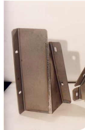
Part obtained by laser welding. Mars® 500 steel
