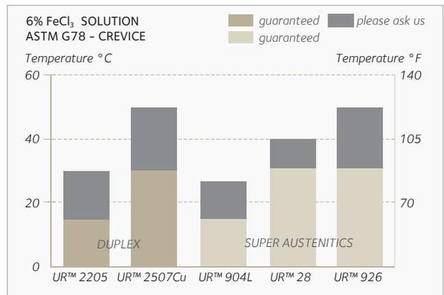
The high chromium, molybdenum and nitrogen contents of alloy UR™ 926 (PREN ≥ 43) explain why the grade is very resistant to localized corrosion even in acidified oxidizing environments. The alloy has been used for seawater applications.
