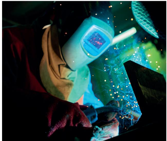
UR™ 926 must be welded with niobium free Ni base filler materials like:
