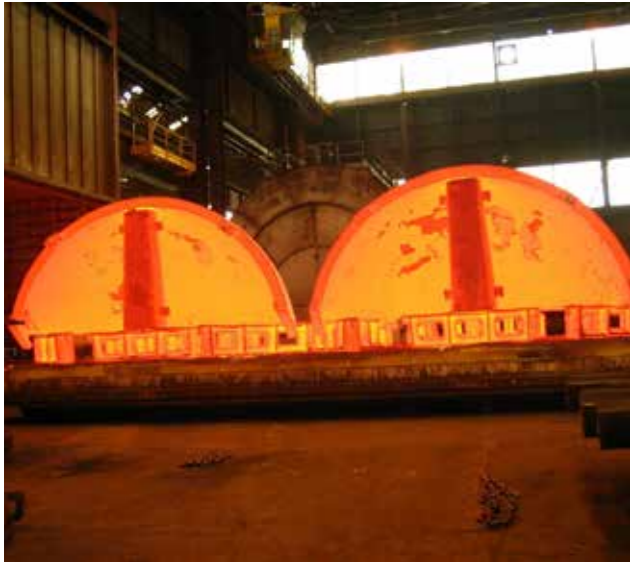
Quality heat treatment on hemispherical 2 piece heads ^
