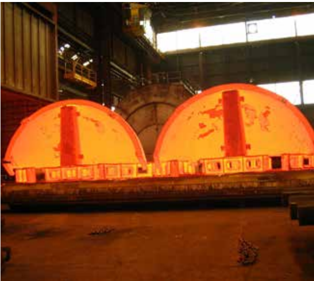
Quality heat treatment on hemispherical 2 piece heads
