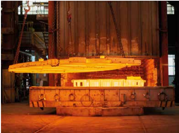
Heating before hot forming ^
