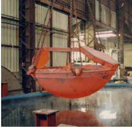
Quenching of formed head ^
