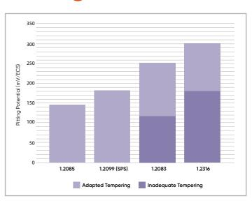
Selecting the mold steel composition is not enough to ensure the righ properties of the steel, the optimal production route is also very important. The corrosion behaviour of stainless plastic mold steels is correlated with the evolution of the microstructure during tempering.
