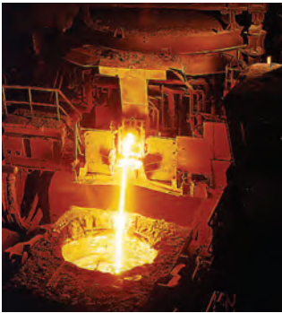
VOD Electric arc furnace ▼
