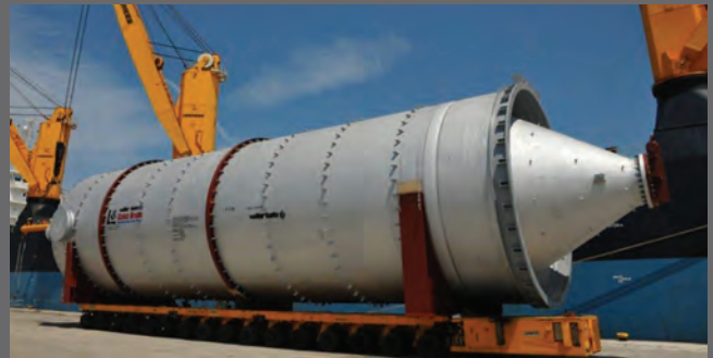
SA387Gr11 backing with 410S cladding ▲
