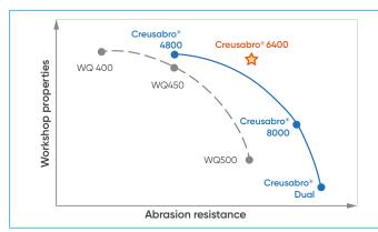
Creusabro® 6400 has been developed to meet all situation where improved wear resistance is required keeping the same formability and easy process-ability in the workshop as classical 450 HB plates.
