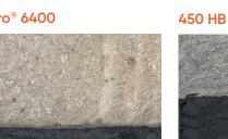
Sample aspect after 2h MLD test, 150 beats (3J)/min, 200 rot/min, Silica flow 7,12 g/s
