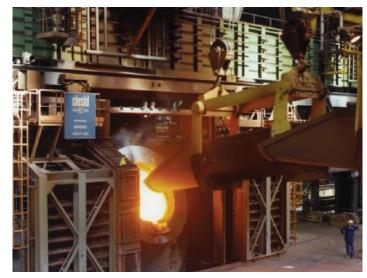
Metal scraps Feeder in ArcelorMittal Fos, use of Creusabro<sup>®</sup> 8000 allows weight reduction and reduce energy consumption
