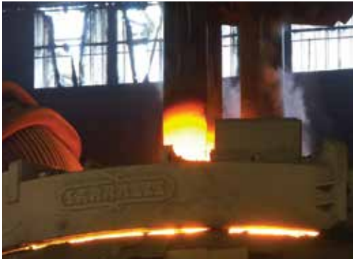
Electric arc furnace (capacity : 90 tons) ▼
