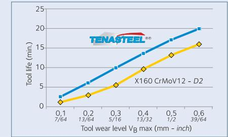
Test on annealed sample
