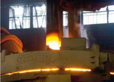
Electric arc furnace (capacity : 90 tons) ▾
