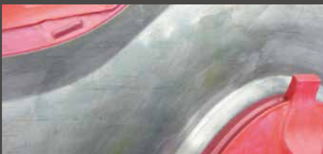
Cavity made of standard P20 + Ni was rejected due to segregation streaks
