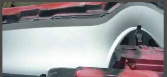
Cavity made of Superplast® P20 was approved by end user
